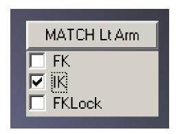
Additionally, there are four Match buttons, each corresponding to a different limb. These will match any of the controls schemes checked off to the current position of the joint chain. This is very useful for when you need to switch between IK and FK in the middle of an animation and don't want any "popping."
